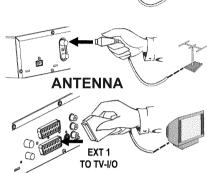
Insert one end of the supplied aerial cable into the TV OUT socket at the back of the DVD recorder and the other end into the aerial input socket of the TV set.
